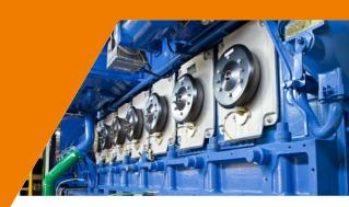
WÄRTSILÄ<sup>©</sup> 32 bore engines have been the preferred choice of yards, operators and owners since the 1980s, with more than 5100 engines delivered to the marine market alone. The Wärtsilä 32 is available with 6 to 16 cylinders and a power output ranging between 3 and 9.3 MW at 720 and 750 RPM. It has best-in-class power density and fuel economy over a wide operating range.
