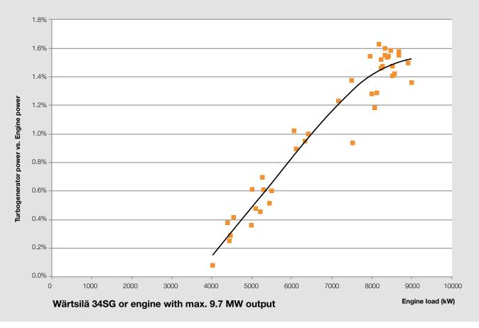
The efficiency of the turbogenerator rises quickly as the engine load is increased.
