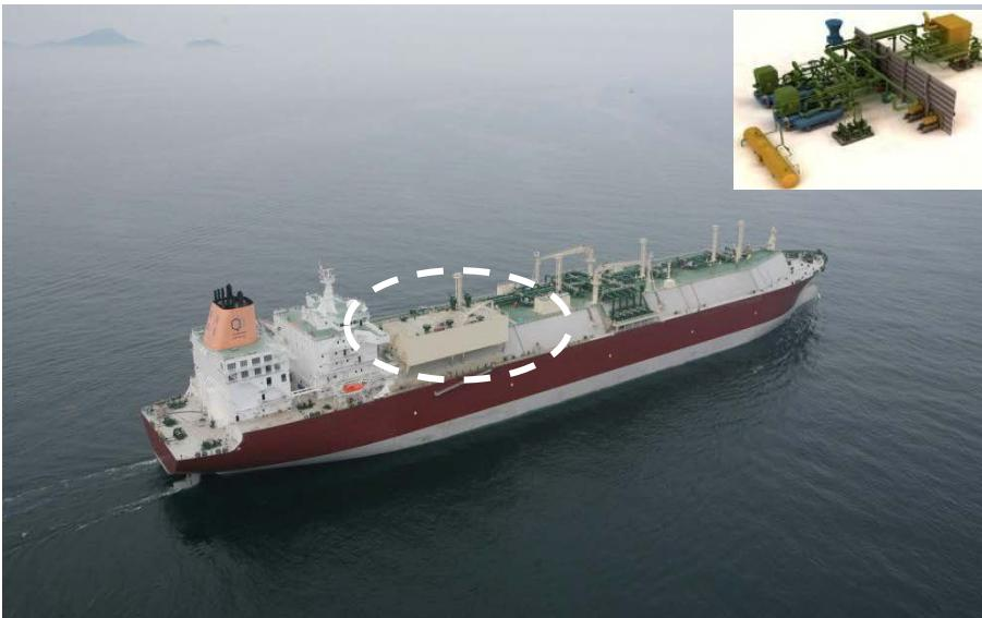
LNG Carrier cargo tank BOG handling
