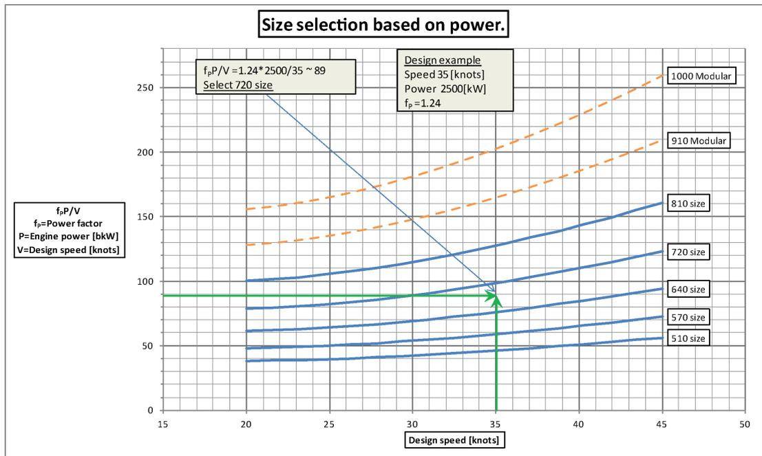
Fig 5-3 Size selection based on power
