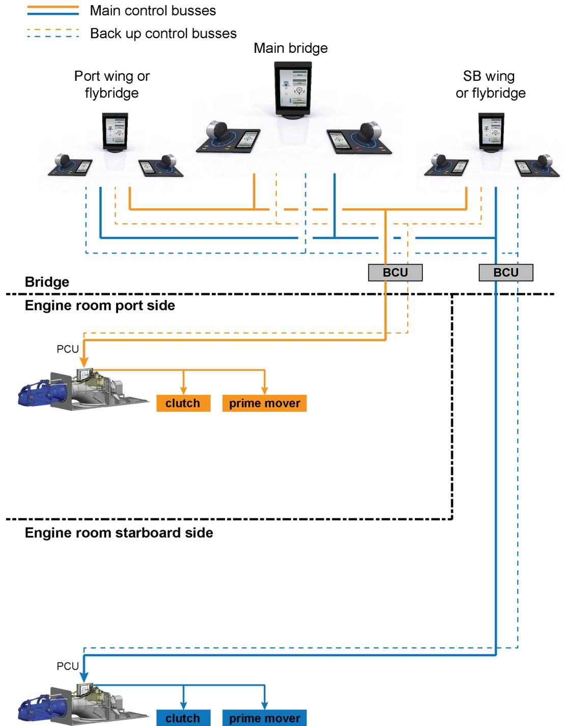
**Fig 7-2 Two steerable waterjet system**
