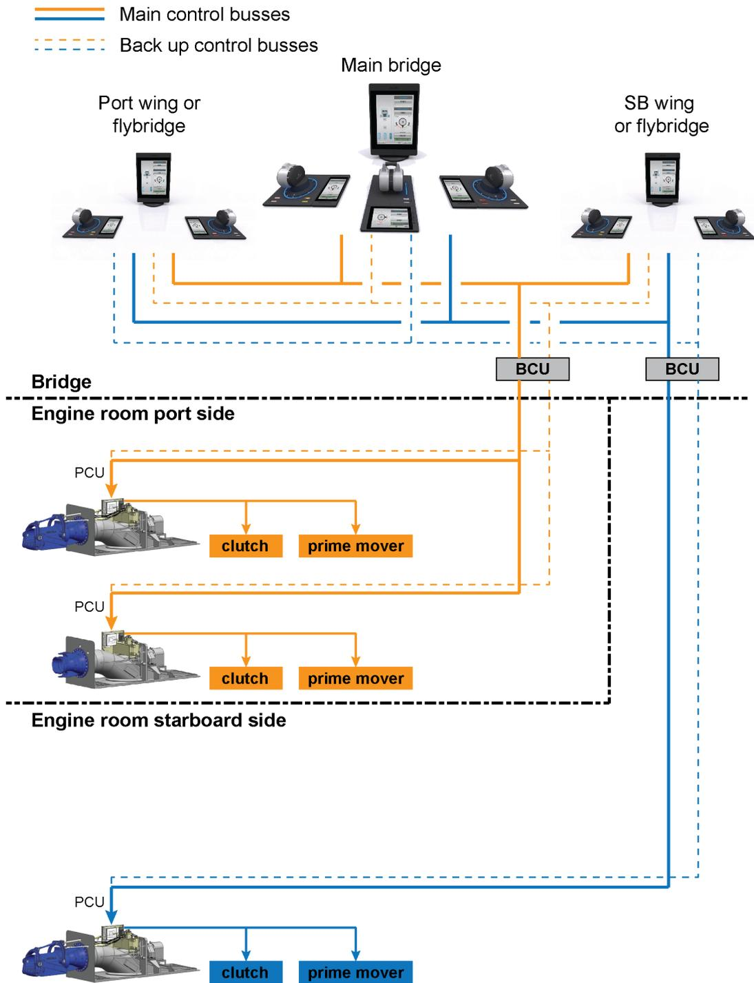
**Fig 7-3 Two steerable and one booster waterjet system**
