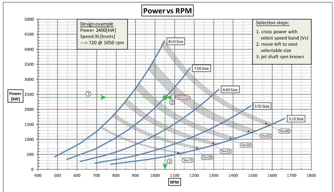
Fig 6-1 Power vs rpm
