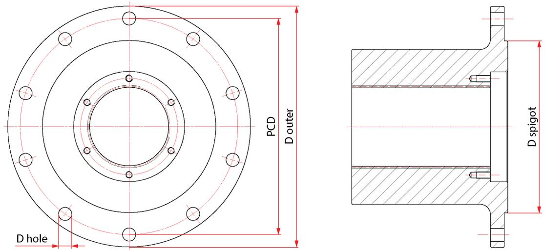
**Fig 6-5 Coupling interface dimensions**
