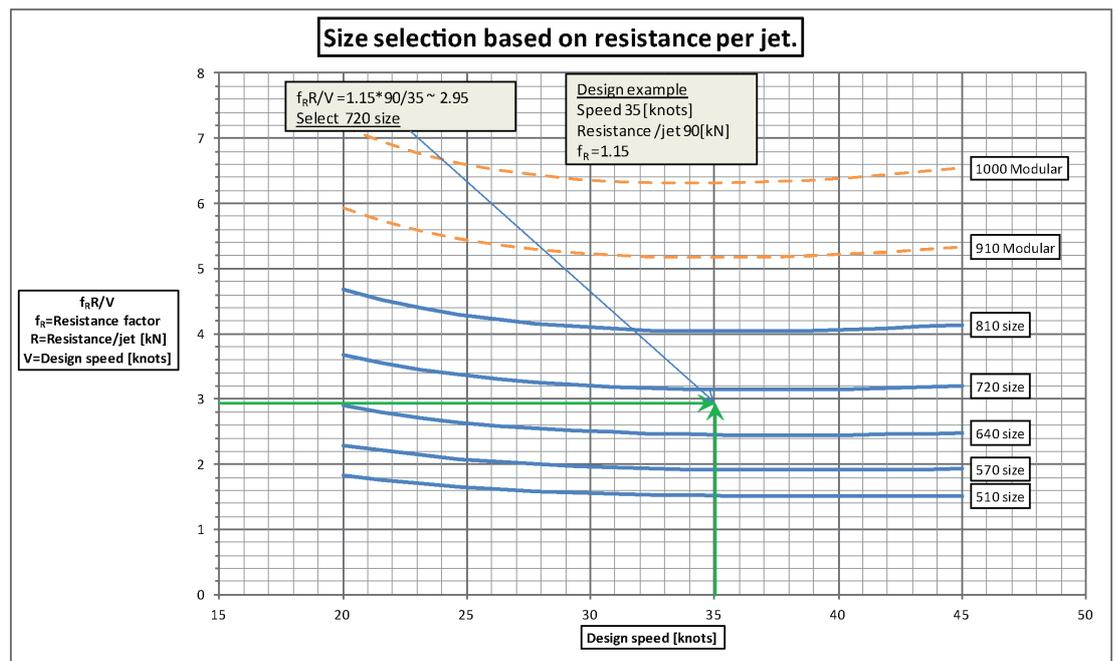
Fig 5-5 Selection based on resistance
