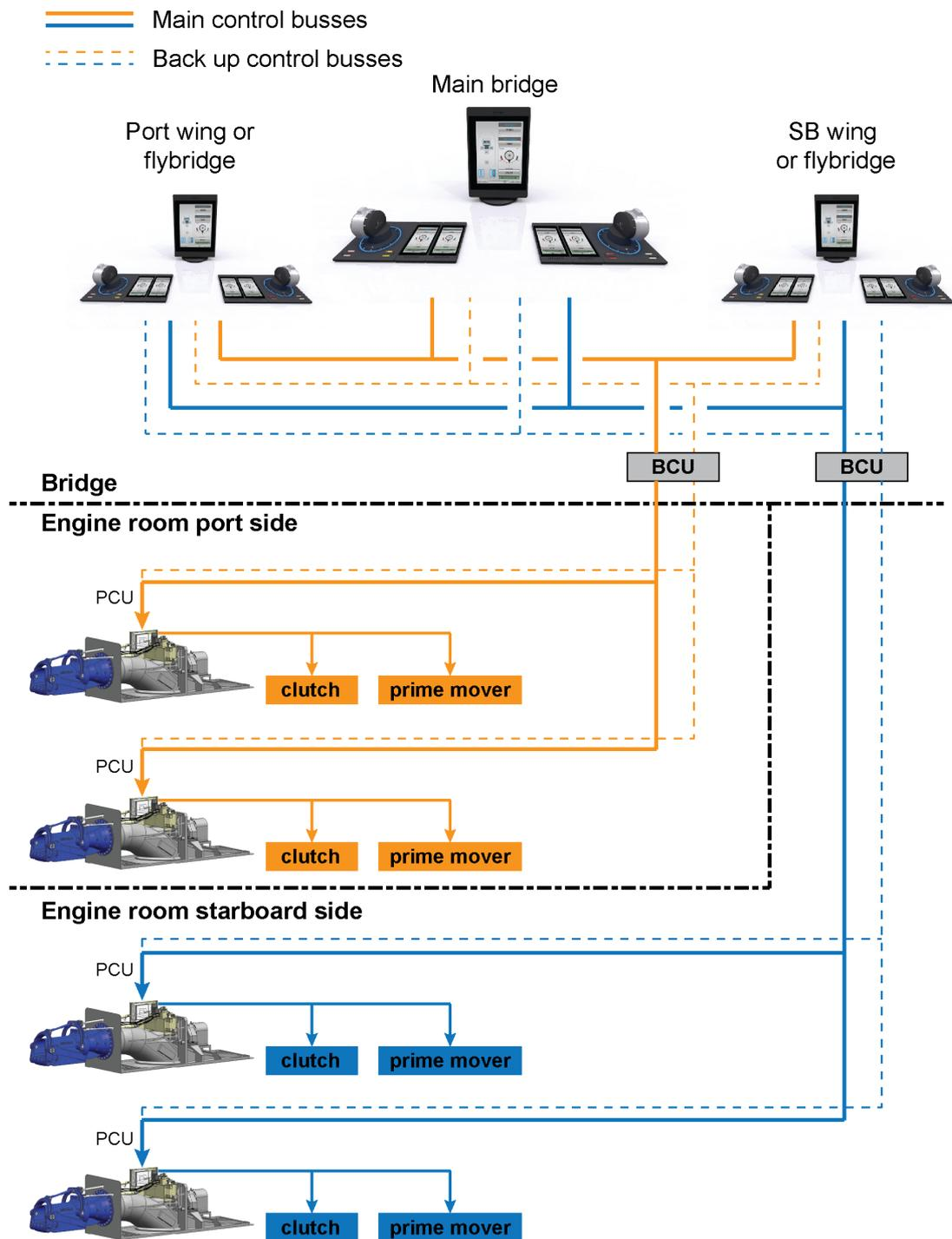
**Fig 7-1 Four steerable waterjet system**
