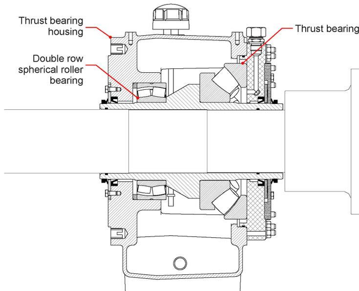
**Fig 4-4 Sectional view of thrust bearing block**
