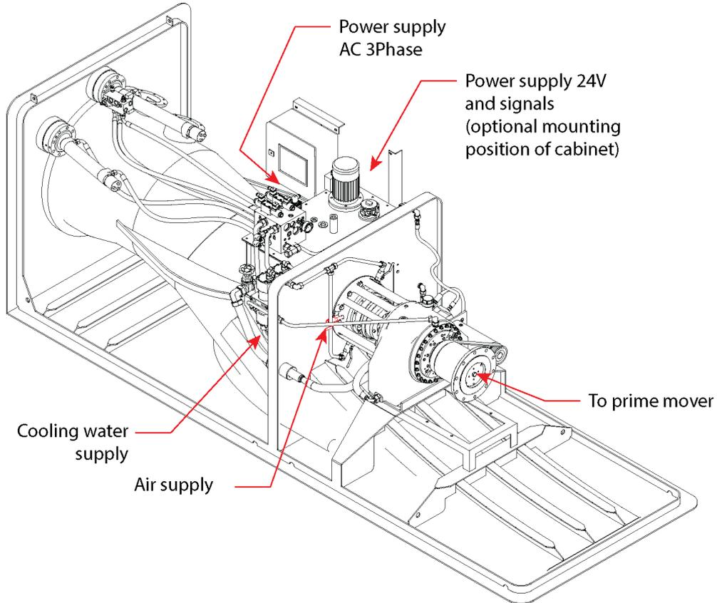
**Fig 6-4** Interfacing connections
