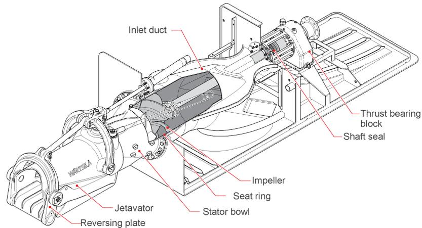
**Fig 4-1 Waterjet with steering and reversing capability**
