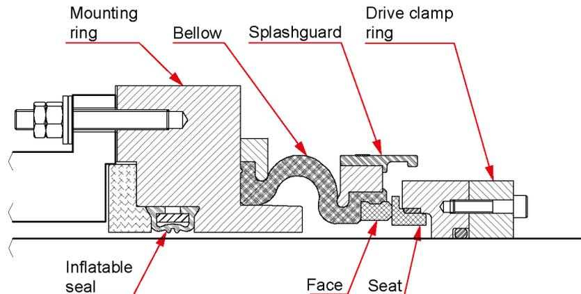
**Fig 4-3 Shaft seal**
